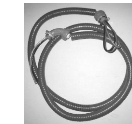
Non-Metallic Power Whip for Outdoor Use (Field-Supplied, Not Spliced and Not Knotted, Water-Proof Sealed Tight, UL Approved)
